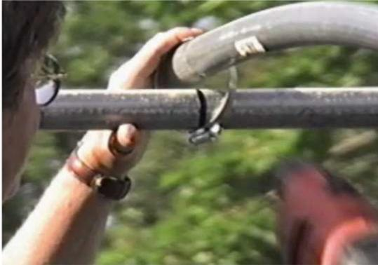
**NOTE: Regular greenhouse purlin clamps can also be used in place of the hose clamps. Our kits come with Purlin Clamps not hose clamps.**
