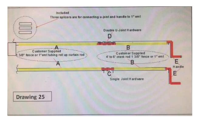
Your roll up curtain rod can be made of 1 3/8" fence tubing (recommended) or 1" emt for shorter houses . Typically the rod length extends between 12' to 16" past each end of the greenhouse then cranking hardware is attached. Self drilling tech screws are supplied to attach hardware to your tubing.
