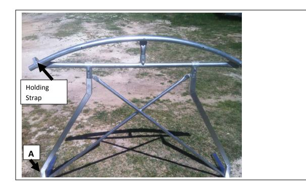
Our vertical leg adapter kit is designed for use with any of our EC- Series benders. The foot denoted in (A) above will require heavy sand bags or other weights when bending hoops to prevent it from lifting off the ground.
