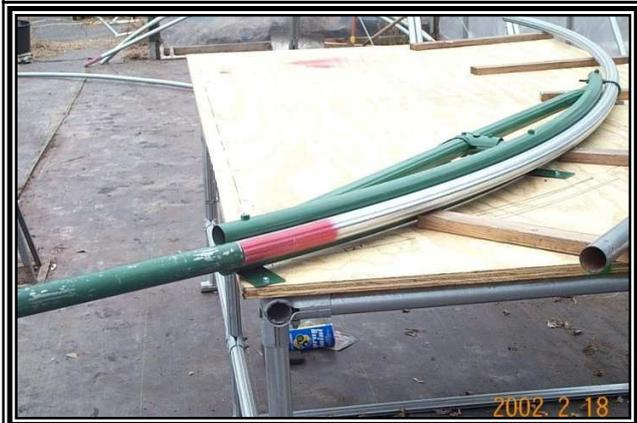
Here I've bent and pushed some of the tubing thru the bender and pulled the more tubing around the bender towards me in this bending stroke. Making sure that the tube I'm bending stays in the groove formed by the twin tube bender body.
