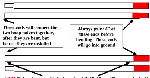
"B" Using factory 21 ft. lengths 1 3/8" 18 or 17 ga. cut in half.
