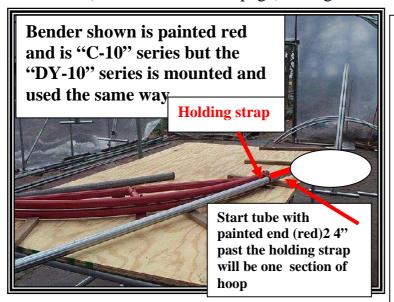
Remember the 10 wide frame is a two piece (section) hoop. The photo at left shows placing one of these 10'6" tubes with large end painted red into bender, When you bend the other half section tube you will push the small end painted (red) through the holding strap twenty four (24") And bend as instructed. When both sections are completed they will join together at the top of the hoop, described later.
