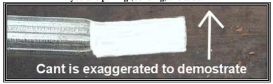
Insert about twenty four (24) inches inches of the tube end indicated by red paint (see tube orientation page) through the holding strap of the bender.
