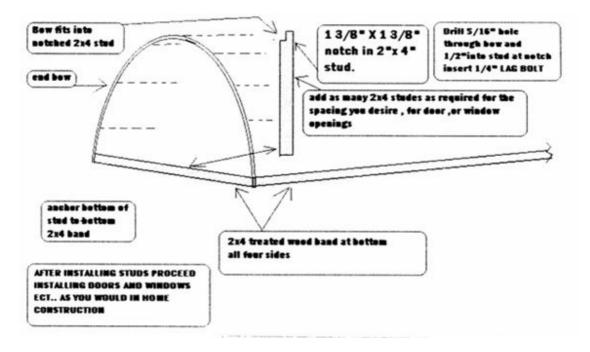
Wood framing is attached to end hoops with a number of different methods, usually simply bolted wit 1/4" carriage bolts or lag screws
