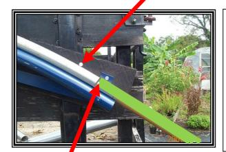
In this photo the junction of the lever bar (GREEN) makes contact with the bender 4" before the junction reaches the end of the bender. The contact point of the Junction can be anywhere on the bender but should never be closer than 4 inches from the end on the bender
