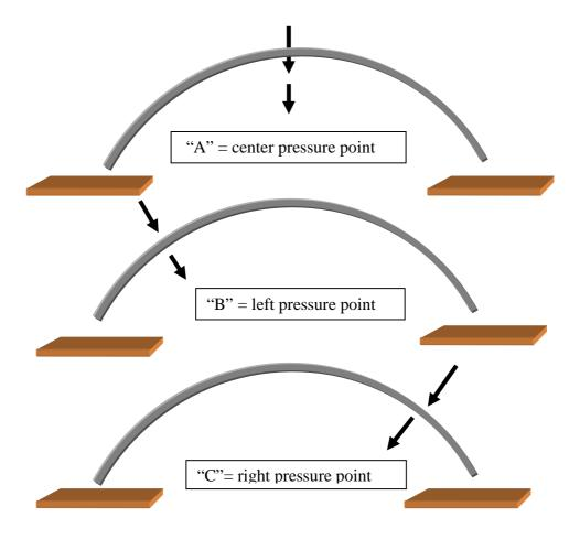
The three pressure points are the same on all 10' 6" long hoop sections. Applying pressure at these three points on each section and by allowing the ends to slide freely when pushing down, each section will uniformly be resized into wider hoops. After a few hoop sections this method will resize a section in about 20 seconds each. AGAIN, NEVER attempt to resize using any other method or press down in more places other than the three points shown above.
