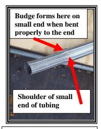
Budge shown above, tubing shown is armadillo Brand tubing and is fluted tubing not smooth as is most.
