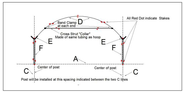
This is how the template is made with the first hoop.
