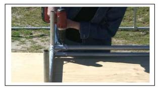
Position the axle carriers close to the first frame from the rear of the tractor but do not tech screw in place. Now slide the 1" emt axle through the top of the carriers. The axle tube must extend 2" past the axle carriers on each side. See close up of position.
